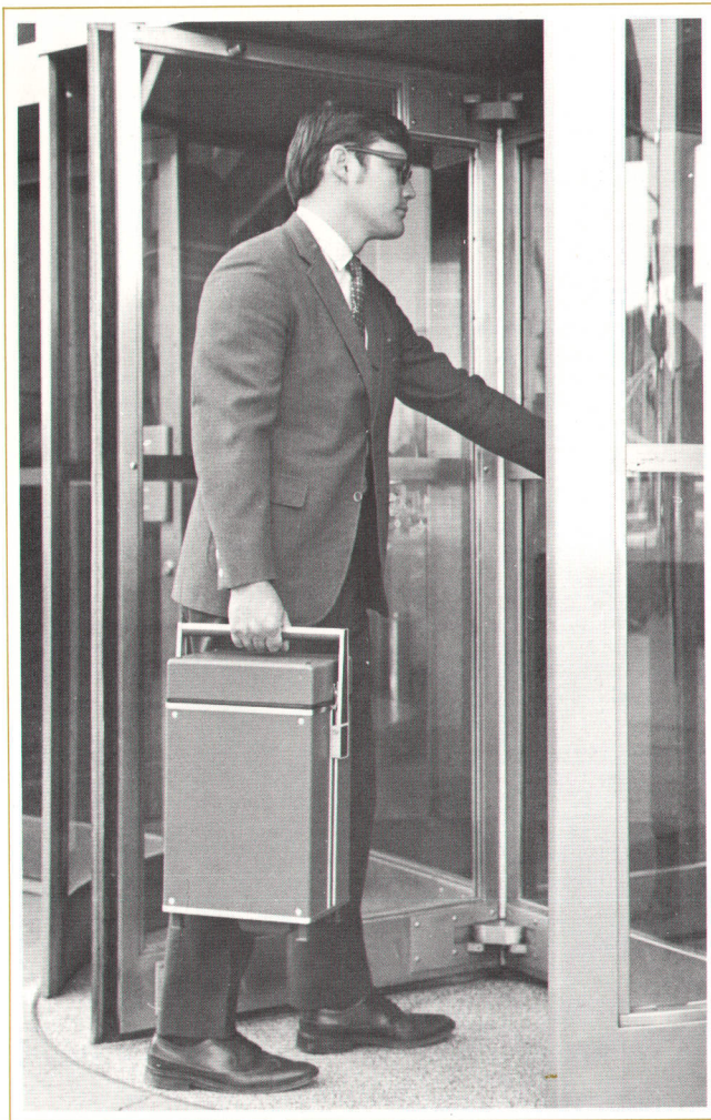
Fig. 8. Oscilloscope's form factor facilitates carrying. Handle locks in three different positions for either carrying instrument or elevating it on a bench for viewing. Snap-on front-panel cover has space for probes, power cord and other accessories.
